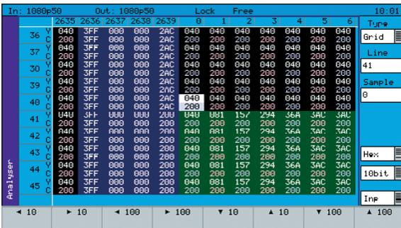
The SDI Data Display & VANC/ANC Inspector option (PHSXOSD) provides the engineer with a detailed view of the data words contained within the SDI stream. This allows the analysis of complex faults and is particularly useful when determining compatibility issues between equipment, and when debugging new product developments particularly in an R&D environment. Detail within the active SDI stream can be viewed with continuous update.
