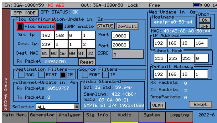
If the SxTAG instrument has the IP 2022-6 Licence option (PHSXO-IP) installed in conjunction with the PHABRIX IP 2022-6 SFP (PHSFP-10SR-IP), it can transmit or receive 2022-6 IP Flows and convert from SDI-to-IP or IP-to-SDI. See the “System - Engineer” section for details on how to control SDI-to-IP or IP-to-SDI Gateway function.
