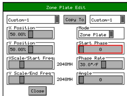
Mode - sets which type of Zone Plate is being produced. It may be Zone Plate (circular pattern) Grating (Linear horizontal or vertical grid) Sweep (Frequency sweeps from start to end Frequency)
