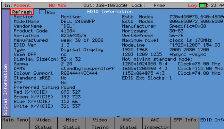
The HDMI EDID viewer option (PHSXO-EDID) displays both RAW ancillary data and decoded EDID information in a tabular display. It obtains the EDID information using a dedicated SFP and cable (PHSFP-HDMI-OUT), which must be purchased separately. For those customers requiring support for 3G formats, an additional license (PHSXO-3GADV) will be needed.
