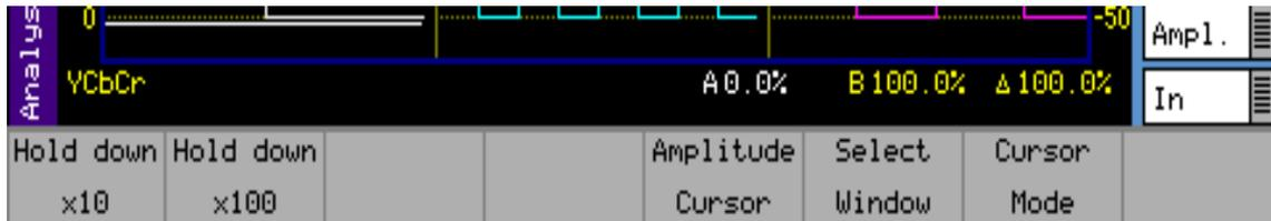
The navigation keys now move the selected cursor around the waveform display which will scroll if moved out of the visible area. The x10 and x100 buttons magnify the action of the navigation keys if held down.
