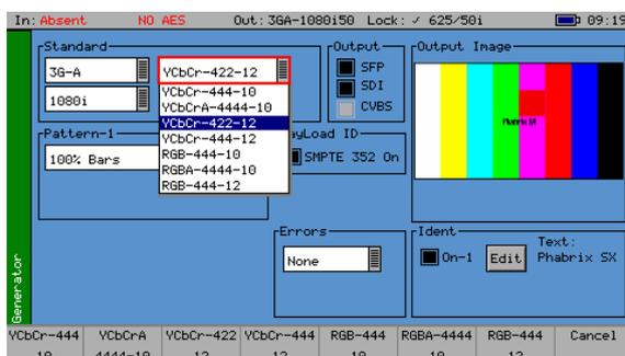
This option (PHSXO-3GADV) provides 3G-SDI Level A and B support including advanced formats: 4:2:2 YUV, 4:4:4 RGB and 4:4:4 YUV at 10/12 bit, and 2K advanced formats including: 4:2:2 YCbCr, 4:4:4 RGB' and 4:4:4 YCbCr at 10/12 bit as well as 4:4:4 XYZ at 12-bit. For broadcast manufacturers this option allows rigorous testing of many more formats beyond the standard signals used in traditional broadcasting.
