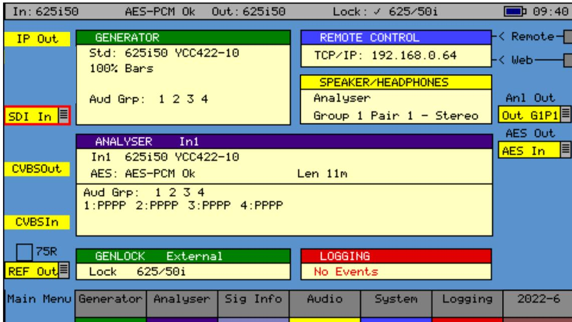
The Main Menu view provides an overview of the system. It shows the video input and output standards and frame rate. The audio status for the generator shows which audio groups are being generated whilst the audio status for the input shows which groups are present and an overview of the channel status for each audio channel.
