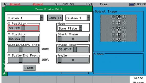
The Advanced Zone Plate Generator option (PHSXOZ) adds a range of preprogrammed zone plate patterns along with user-defined controls over several parameters which can be saved to custom buffers.
