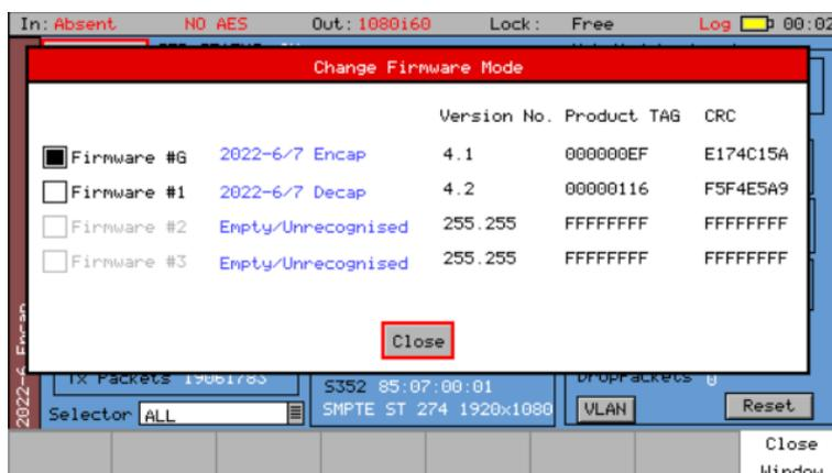
The current SFP firmware mode will be displayed. To change mode, select the checkbox next to the mode required.
