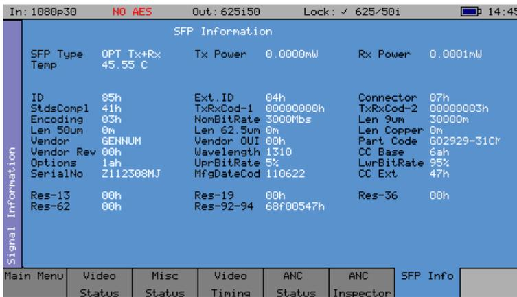
The SFP Info menu displays details of the currently installed SFP module.
