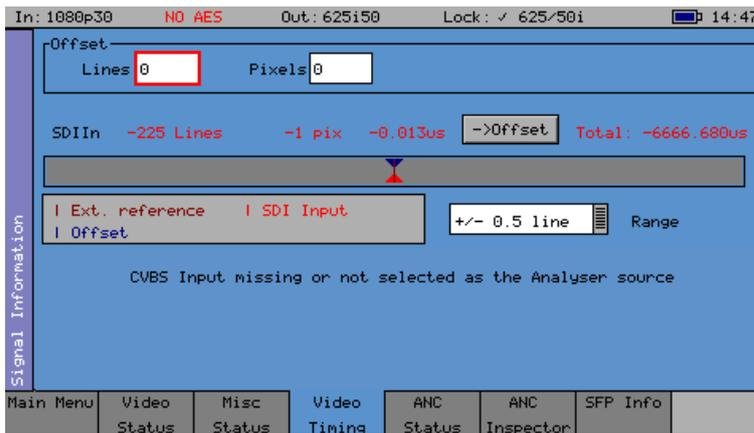
The Video Timing menu displays the relationship between the chosen input (SDI, SFP, or composite) with respect to the locking reference input.
