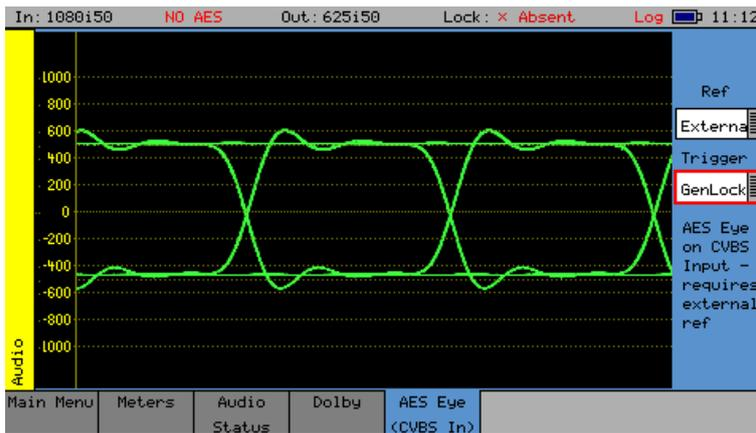
AES Eye menu allows an AES signal of 75Ω impedance connected to the “PAL/NTSC (AES Eye) In” BNC connector to be displayed as an Eye pattern. This allows the amplitude and quality of the AES waveform to be seen and allows, AES to reference locking, to be checked.
