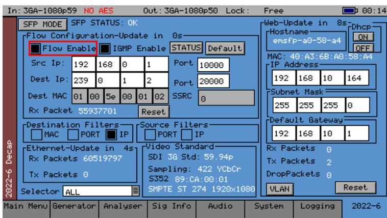
If the SxTAG instrument has the IP 2022-6 Encap/Decap Licence option (PHSXO-IP) installed along with the IP 2022-6 SFP (PHSFP-10SR-2022) it can receive a 2022-6 IP flow.
