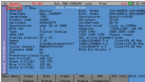
The HDMI EDID viewer option (PHSXO-EDID) displays both decoded EDID information and RAW ancillary data in a tabular display. It obtains the EDID information using a dedicated SFP and cable (PHSFP-HDMI-OUT), which must be purchased separately. For those customers requiring support for 3G formats, an additional license (PHSXO-3GADV) will be needed.
