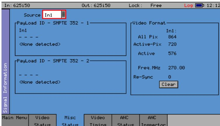
The Misc Status menu displays the status the SMPTE 352 packets embedded in the selected video input, and displays any errors that have been found.
