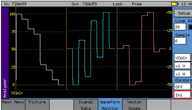
The Waveform menu displays the selected input in the form of a waveform monitor.
