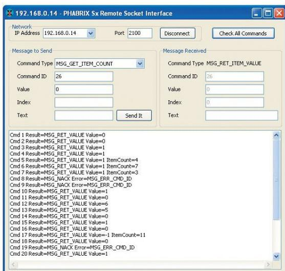
The Enhanced remote control option (PHSXOR) gives users full remote control of the unit via TCP/IP Sockets to allow any aspect of the unit to be modified or queried.
