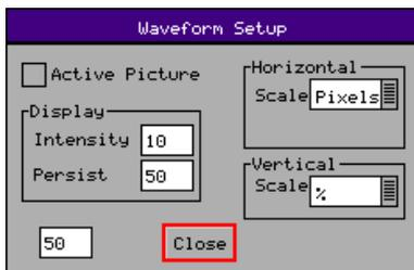
The Waveform Setup menu allows the vertical and horizontal scale of the waveform display to be set up, as well as controlling the intensity and persistence of the display.
