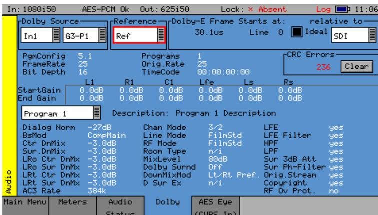
The Dolby-E status option allows display of the Dolby-E metadata present in the selected audio stream and determines whether the Dolby-E packet is timed correctly on the SDI video stream.
