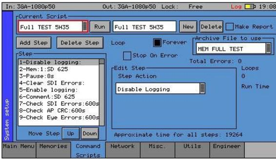
The Command Script & Reports option (PHSXOS) allows a series of predefined actions to be run through within the PHABRIX Sx using a script stored in internal memory.
