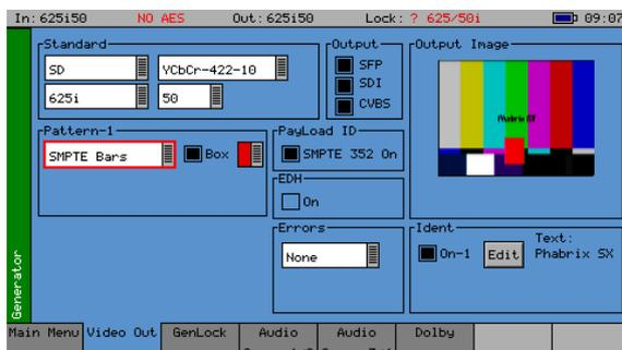
The Generator option (PHSXO-GEN) allows the creation of video test signals for analogue composite video, SD-SDI and HD-SDI video as standard; additionally, 3G-SDI (inc. Advanced formats) & 2K SDI, and Fibre video functionality too, if these options have been purchased. The Generator option also allows the generation of both analogue and digital audio test tones and allows the unit to be locked to an external locking reference.
