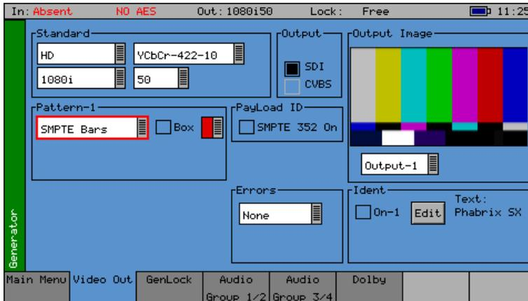
If the SxTAG instrument has the Generator option (PHSXO-GEN) installed it can create video test signals for all supported SD and HD SDI output standards including the 3GHz standards at 1080p/50/59/60. It will support Y,Cr,Cb formats as well as RGB formats.
