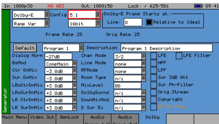
The Sx instrument Dolby bit-stream Analyser & Generator software option (PHSXO-DAG) allows generation of Dolby-E, Dolby Digital and Dolby Digital Plus pre-encoded test signals to check that they are transferred transparently through the broadcast chain unaffected by routers/switchers, satellite links, etc.
