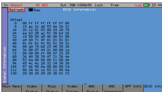
Additionally, the HDMI EDID display option can be used in conjunction with the generator, providing an SDI pattern which is generated through the HDMI SFP which can be used to test a monitor display.
