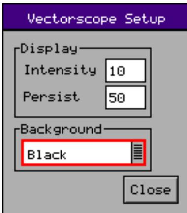
The Vectorscope Setup menu allows the intensity and persistence of the display to be adjusted. A colour wheel background can also be added.
