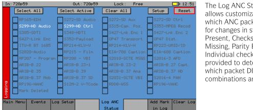
The Log ANC Status menu allows customization of which ANC packets to log for changes in status (e.g. Present, Checksum Error, Missing, Parity Error). Individual checkboxes are provided to determine which packet DID/SDID combinations are logged.
