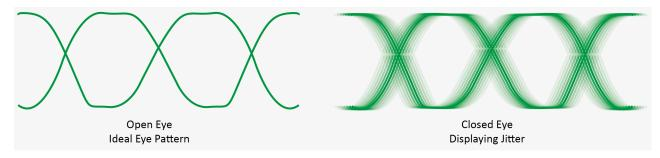
The Eye Pattern is formed by displaying the clock signal from the SDI data stream then superimposing a delayed version of the clock signal at exactly halfway through the duty cycle (or unit interval) of the clock signal, forming the recognizable eye shape.
