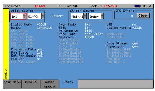
When Dolby Digital Plus metadata is analyzed, this displays the Main, Dependent and Independent program stream configuration and limited metadata that is sent with Dolby Digital Plus.
