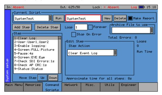
The **Command Scripts** menu allows the Sx instrument to run predefined scripts. This can be used to automate testing of signals.
