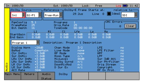
This displays the Program configuration (5.1+2 etc.), the number of programs in the metadata, the frame rates and bit depths and timecode if present.
