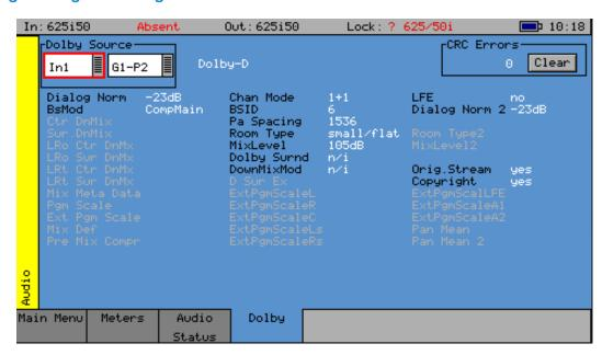
When Dolby Digital metadata is analyzed this displays channel configuration and limited metadata that is sent with Dolby Digital.
