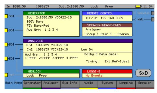
The Main Menu provides an overview for the system. It shows the video input and output standards and frame rate. The audio status for the generator shows which audio groups are being generated whilst the audio status for the input shows which groups are present and an overview of the channel status for each audio channel.
