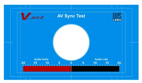
The LAWO V\_line AV Sync test pattern provides a constantly moving progress bar. When the progress bar reaches the center frame of the test pattern, first a vertical white bar then a white flash appears in the center circle.
