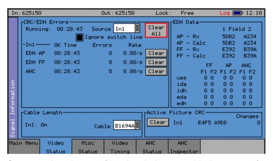
The Video Status menu shows the status of the selected video input and displays any errors found in the datastream.
