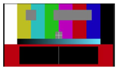
The Sx modified EBU Tech 3305 AV Sync test pattern provides a constantly moving clapperboard that when it closes shows a vertical white flash line for one frame.
