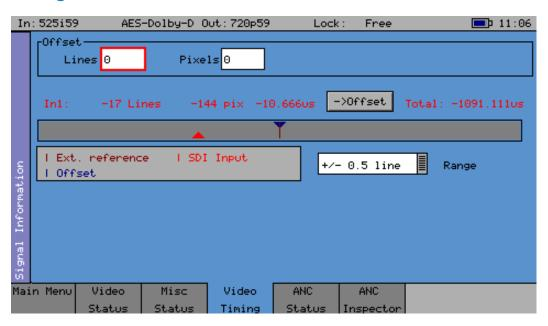
The Video Timing menu displays the relationship between the selected video input with respect to the locking reference input.
