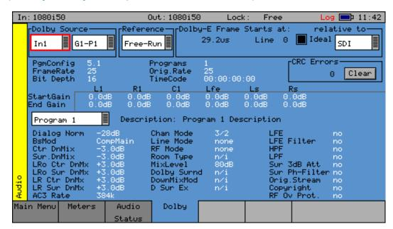
The **Dolby** Analysis option allows display of the Dolby E metadata present in the selected audio stream and determines whether the Dolby E packet is timed correctly on the SDI video stream.
