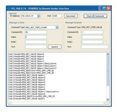
The Enhanced Remote Control Integration option (**PHSXOR**) gives users full remote control of the unit through TCP/IP Sockets to allow any aspect of the unit to be modified or queried.
