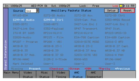
The **ANC Status** menu shows which ANC packets are present on the SDI input and whether they have any errors. Each field is color-coded according to whether the ANC packet is present (White), missing (Grey), has errors (Red), or has previously had errors (yellow).
