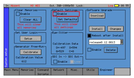
The **Engineer** menu is used to manage the unit and allows user access to be setup and the installation of new versions of software.
