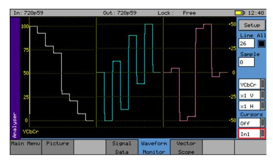
The Waveform Monitor menu displays the selected input in the form of a waveform monitor.
