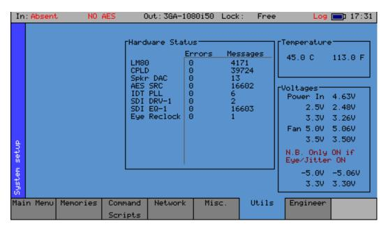
The **Utils** menu displays details of the instrument's operating status and displays the temperature and individual voltages. This menu also allows you to disable selected options.
