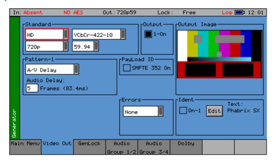
The AV Delay Generator produces an adapted EBU Tech 3305 AV Sync *clapperboard* Test Pattern. An audio delay offset with respect to video of up to +/- 40 frames can be applied in increments of one frame.
