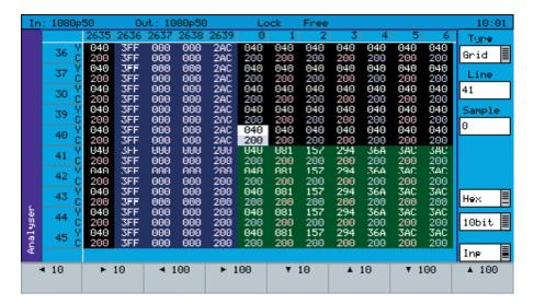
The SDI Data Display and VANC/ANC Inspector option (**PHSXOSD**) provides the engineer with a detailed view of the data words contained within the SDI stream. This allows the analysis of complex faults and is particularly useful when determining compatibility issues between equipment and when debugging new product developments particularly in a research and development environment. Detail in the active SDI stream can be viewed with continuous update.
