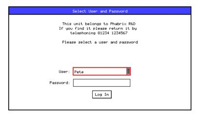
Using the User Login feature allows the Sx to be protected from unauthorized operation of the Front Panel controls. The prompt feature can allow a message to be displayed so that if the Sx instrument gets lost or stolen, someone finding it knows where to return it.
