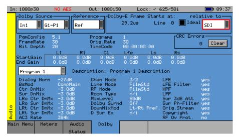
The Dolby audio may be monitored from any of the SDI input embedded audio channel pairs. Peak audio levels are also displayed for Dolby E.
