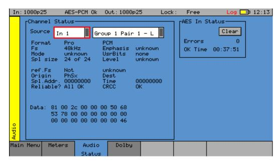
The **Audio Status** menu shows the Channel Status for the selected audio channel displayed in decoded form as well as a hexadecimal dump of the bytes. The source may either come from the input signal or from the generator for comparison purposes.
