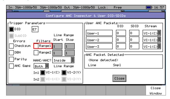
If the **Setup** button is pressed a dialog box allows the ANC packet trigger parameters to be set. The trigger parameters allow only selected lines to be checked or excluded when checking for the presence of packets.
