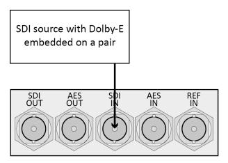
In this example, the SDI signal contains embedded audio with Dolby E present on one or more audio pairs. The Sx instrument needs to lock its internal audio clock to the SDI signal **Generator → GenLock** → **GenLock Source → Input-1** and the Dolby Timing source should be set to **SDI**.
