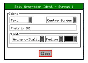
The **Edit Generator Ident** dialog allows selection of either a user-defined bitmap picture, downloaded into the **Idents** directory of the Sx instrument or user-defined text.
