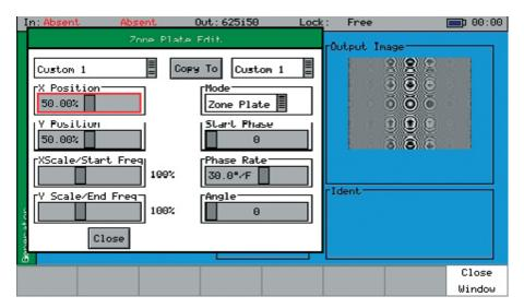
The Zone Plate Generator option (**PHSXOZ**) adds a range of preprogrammed zone plate patterns along with user-defined controls over several parameters which can be saved to custom buffers.
