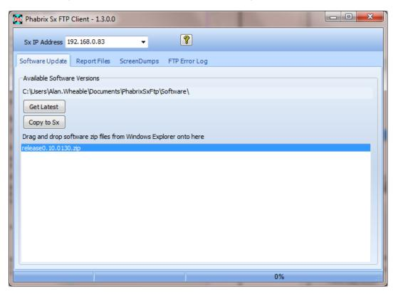
To connect to the instrument, you will need to use the PHABRIX FTP client available from the PHABRIX website. This connects to the Sx unit using IP address of the unit (as host name) with:
