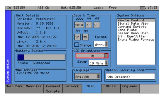
The **Misc.** menu shows serial numbers, Sx instrument MAC address, version information and battery state. It also allows the date and time to be set and factory default settings to be recalled. The **Options Security Code** is entered on this page to activate purchased options.
