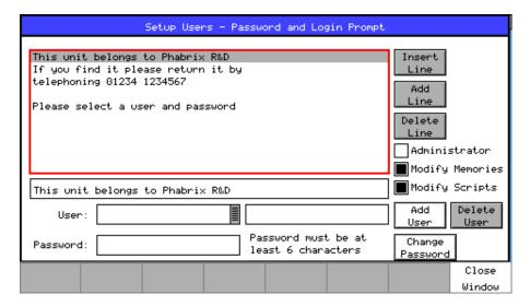
Once user login has been set up on your Sx a **Log out** button is added to the main menu which displays a Login screen. This may be used to protect systems settings from being modified by other users. The system is still operating while the login screen is visible.
