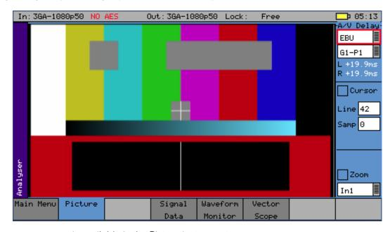
AV Delay measurement is available in the Picture instrument.
