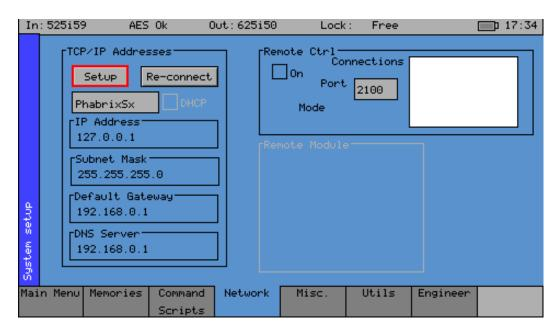
PHABRIX Sx is fully network compatible and has a complete network interface to allow control of any Sx instrument from any other unit.
