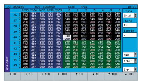
The SDI Data Display and VANC/ANC Inspector option (**PHSXOSD**) provides the engineer with a detailed view of the data words contained within the SDI stream. This allows the analysis of complex
