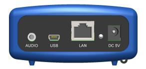
The Sx instrument Control panel provide the following connections.
