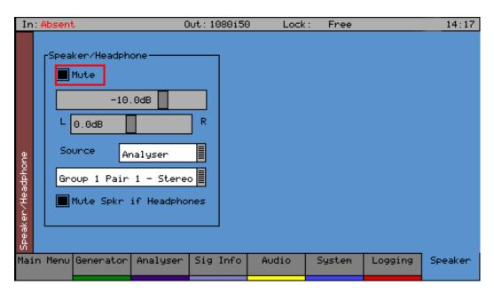
The **Speaker** menu controls which audio pair can be heard on the loudspeakers and headphone output of the Sx instrument. The Sx instrument contains a stereo loudspeaker and associated stereo headphone socket which can be connected to any of the audio input or output channels or pairs.
