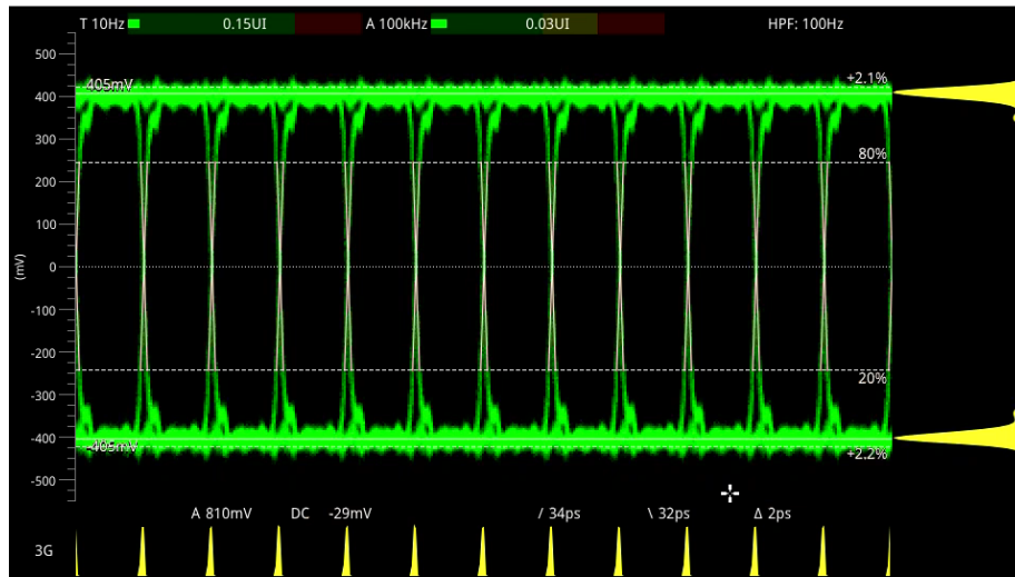
Figure 13-2: 3G-SDI Eye Pattern Set to Display 12 Eyes (Using Green Display Color)
