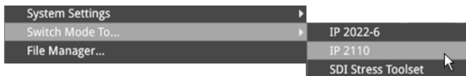
Figure 3-15: Switching Between Qx Boot Modes
