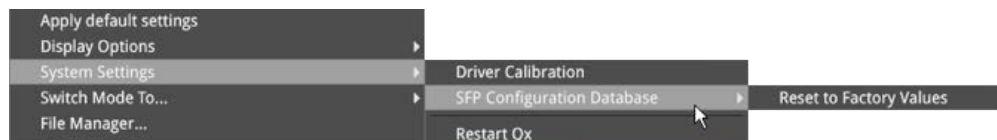
Figure 3-19: Resetting the SFP Configuration Database
