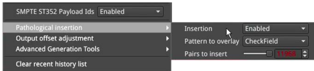
Figure 6-9: Generator - Pathological Signal Insertion Options
