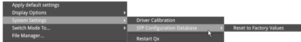
Figure 3-19: Resetting the SFP Configuration Database
