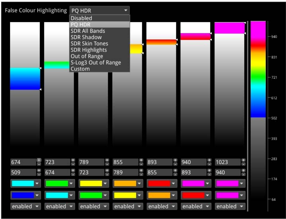
Figure 15-5: Configuring the False Color Overlay
