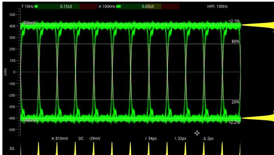
Figure 13-2: 3G-SDI Eye Pattern Set to Display 12 Eyes (Using Green Display Color) (SDI Boot Mode)
