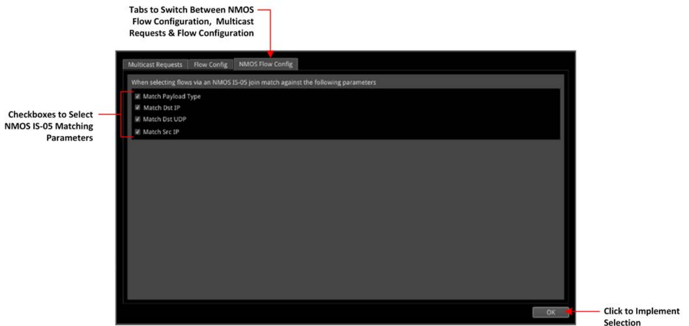
Figure 4-34: IP Receive - Flow Select: NMOS Flow Config Tab
