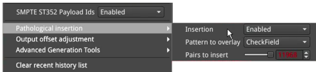
Figure 6-9: Generator - Pathological Signal Insertion Options
