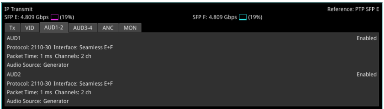
Figure 6-18: IP Transmit - AUD1-2 Status Tab
