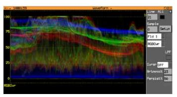
Individual video line selection can be made which can be useful to view the levels on specific lines
