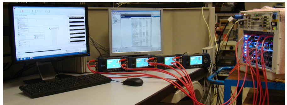
Figure 6. Quantel sQ Server under test using PHABRIX SxE T&M instruments
