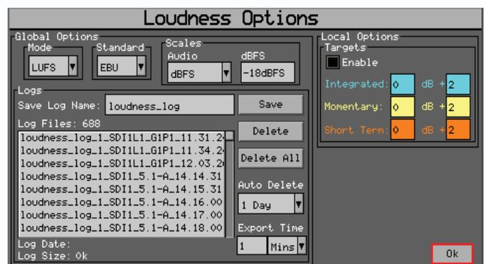
The “Integrated”, “Momentary” and “Short Term” threshold values define the level, above which, a loudness error is logged as exceeding the defined upper limits. The errors count is displayed on the Loudness window as well as being time-stamped in the log file.
