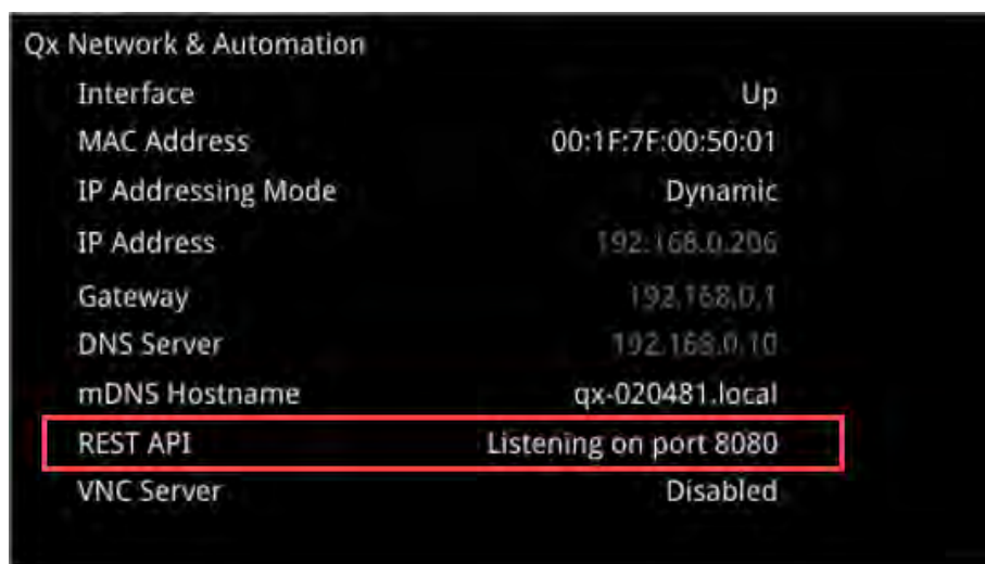
Figure 16-1: REST API Enabled in Network & Automation Window
