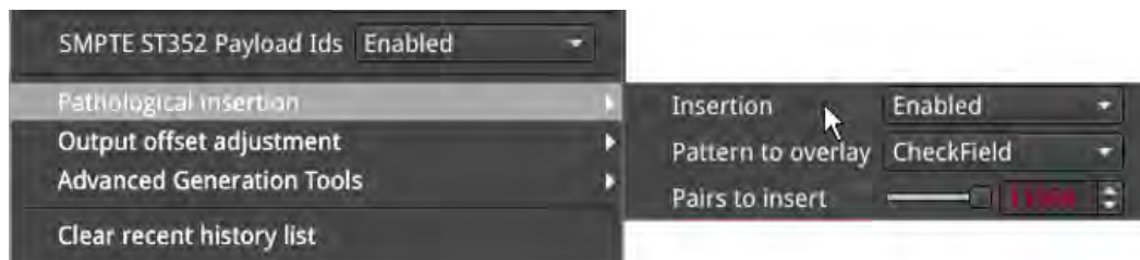
Figure 6-15: Generator - Pathological Signal Insertion Options
