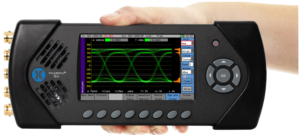
Figure 2. Shows the Eye Pattern displayed on the PHABRIX SxE handheld instrument.
